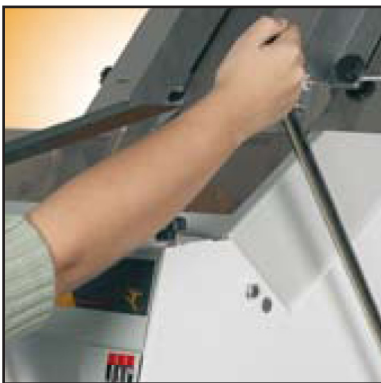
The traction lever helps push the last loaf into the slicing blades.
