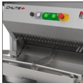
Adjustable bread holder adjusts pressure on the bread to ensure a clean & precise cut.
